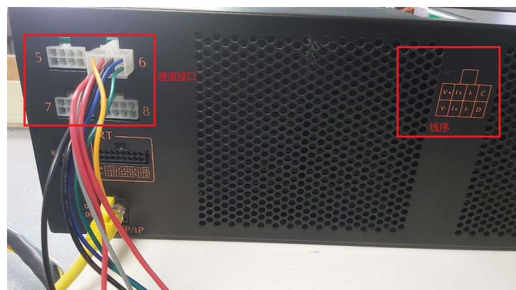
Figure 2-10 Channel wire connection
